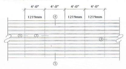
Continuous Louvre of Precoated Steel prebent to size and of ultra violet resistance quality.
